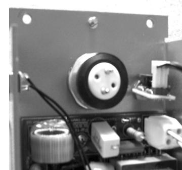
7. Insert new lamp into socket.
